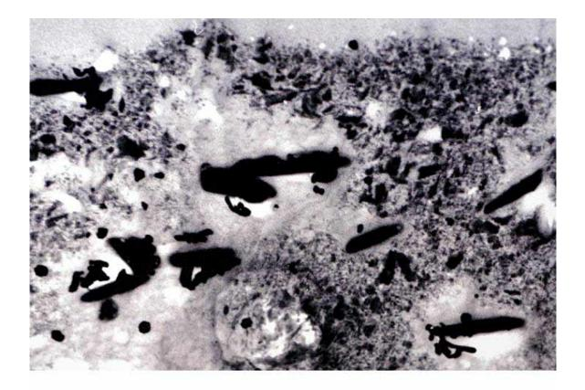
*Figure 5.* Electron micrograph of a photothermographic reversal system layer showing sphere of development inhibition resulting from the release of 1-phenyl mercaptotriazole as a function of physical development. This produces a second stage of chemical development amplification when the system is driven into fog by extended thermal development.
